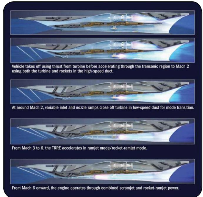
Vehicle takes off using thrust from turbine before accelerating through the transonic region to Mach 2 using both the turbine and rockets in the high-speed duct.
