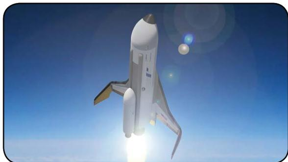
The winged XS-1 spaceplane, dubbed Phantom Express by Boeing, will be powered by the Aerojet Rocketdyne AR-22, a derivative of the rocket company’s RS-25 space shuttle main engine.
